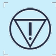
Figure 2 - Symbol IEC 60417-5638: Emergency stop
