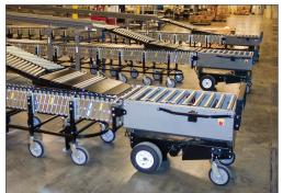
The PowerTrax takes the work out of moving conveyors in and out of trucks for faster, easier and safer while loading and unloading trucks. Simply press the forward button and the PowerTrax will pull your conveyor into a truck. Press the reverse button, and the PowerTrax will push your conveyor back out to the loading dock floor.
