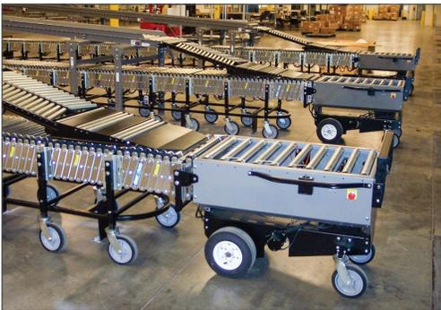
The chasis is all-bolted 10 gauge steel. A strong positive traction running gear pulls the 12" tired for easy traveling over dock levelers. No special wiring is required. Operates on 110 volts. Available with powered roller bed or gravity bed.
