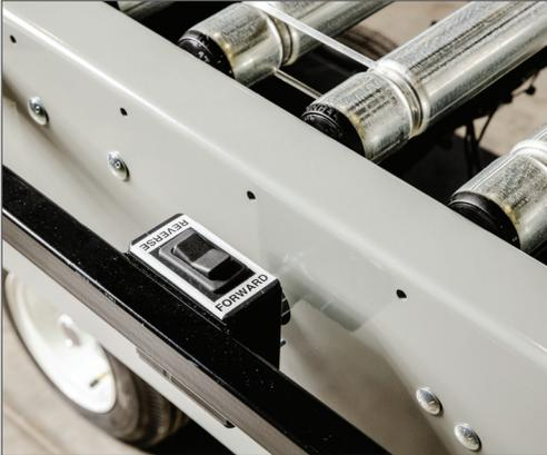
The PowerTrax takes the work out of moving conveyors in and out of trucks for faster, easier and safer while loading and unloading trucks. Simply press the forward button and the PowerTrax will pull your conveyor into a truck. Press the reverse button, and the PowerTrax will push your conveyor back out to the loading dock floor.
